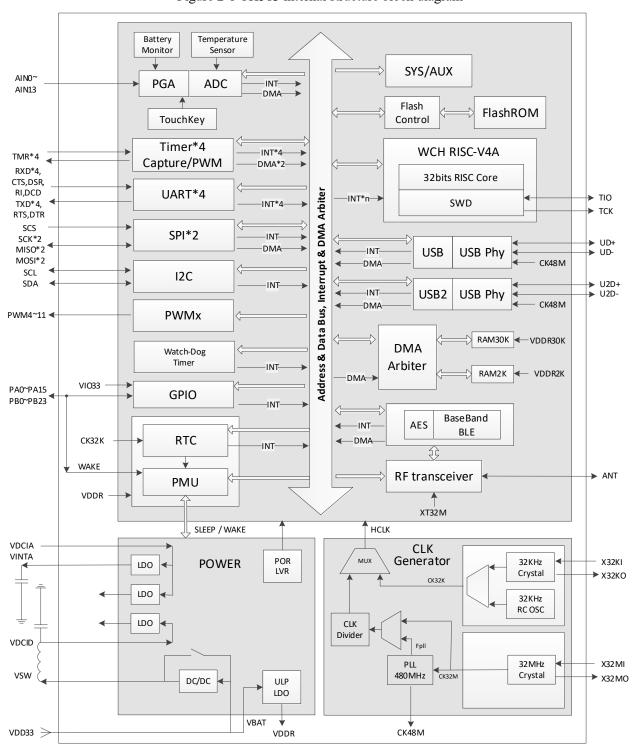
Figure 2-1 CH583 internal structure block diagram
