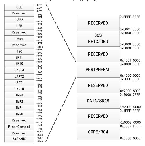
Figure 2-2 Memory mapping diagram
