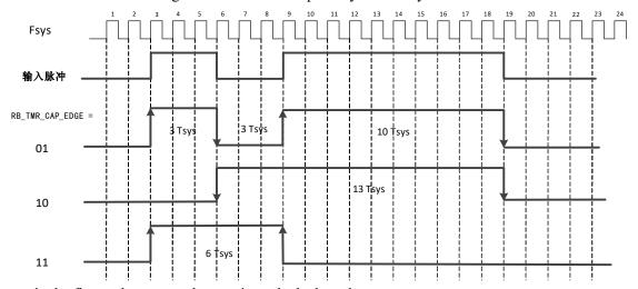
Figure 8-2 Count the capture cycle with system clock
