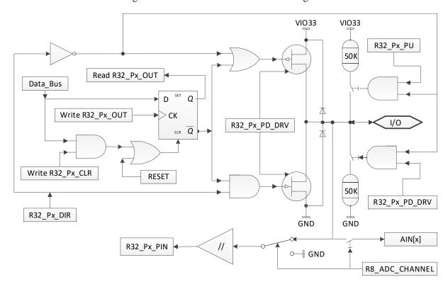
Figure 7-1 I/O internal architecture block diagram
