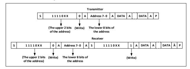
Figure 12-3 Master transceiver data in 10-bit mode
